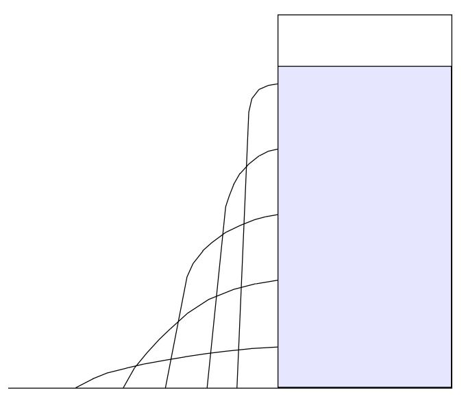
APPARATUS IS APPROXIMATELY 10" SQUARE WITH 5 EQUALLY SPACED HOLES.
