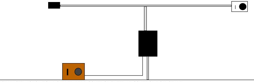
USE "FAST" MOTOR FOR DOPPLER ARM. CONTROL SPEED AT CONTROL BOX. START OUT SLOW THEN SPEED UP.
