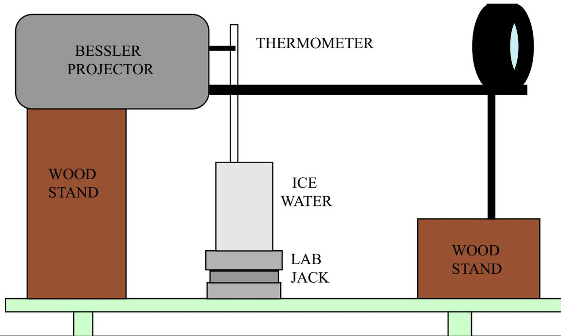
USE LARGE PROJECTOR THERMOMETER ATTACHMENT FOR BESSLER.
