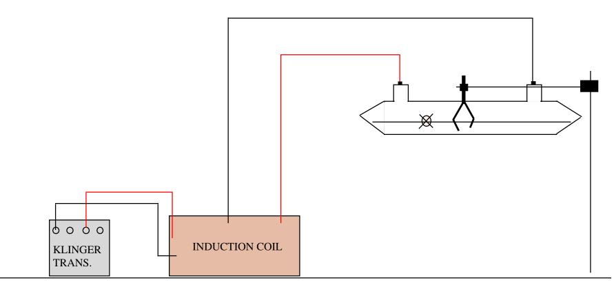
SECURE CATHODE RAY TUBE FIRMLY WITH THREE FINGER CLAMP.
