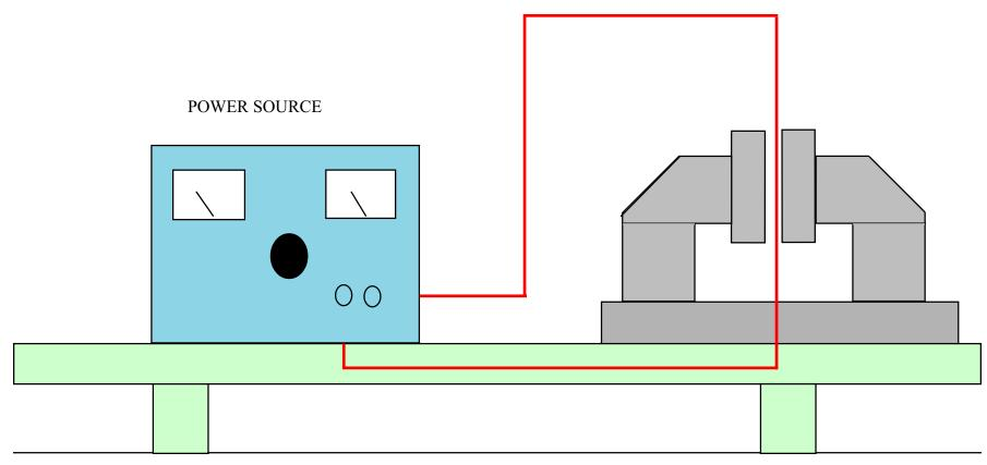
RUN A SINGLE WIRE FROM POWER SOURCE THROUGH MAGNET AND BACK TO POWER SOURCE.
