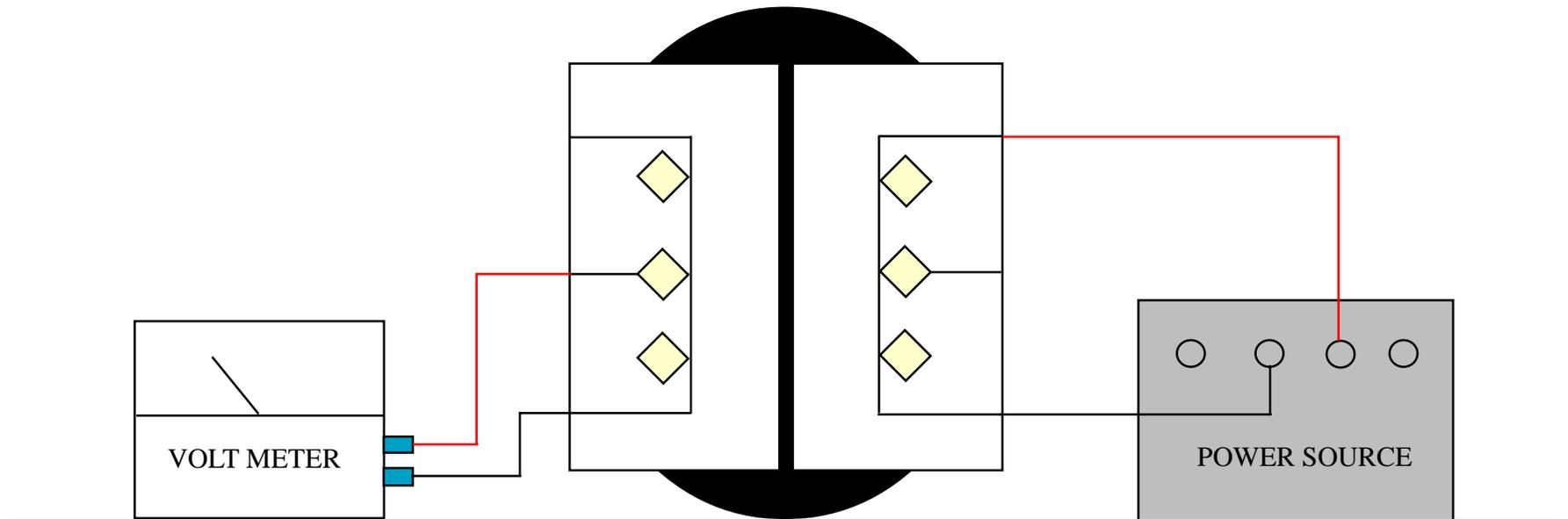
CONFIGURATION OF TRANSFORMER CAN BE CHANGED EITHER BY CHANGING WIRING POSITIONS OR BY CHANGING INSERTS.
