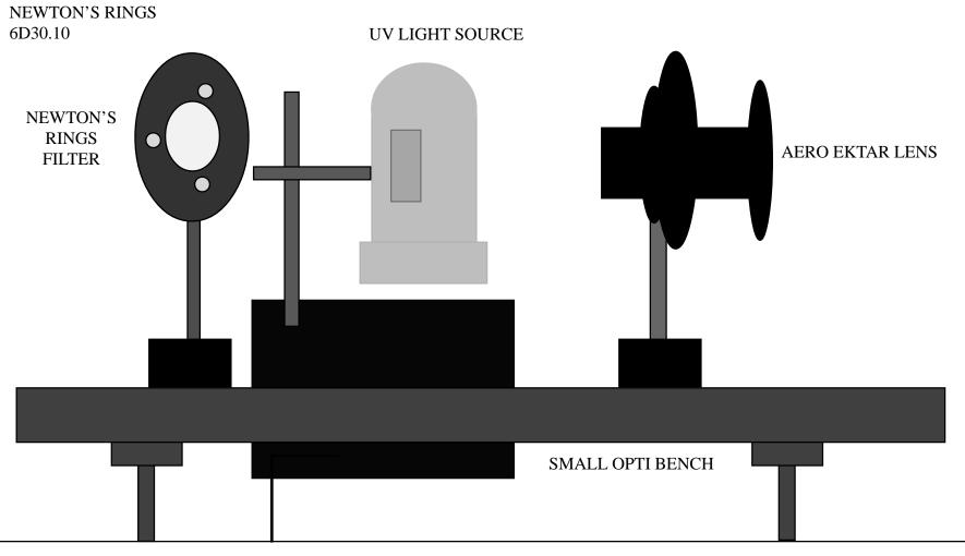
PLACE UV LIGHT SOURCE ~ 3 INCHES FROM THE NEWTON'S RINGS APPARATUS.
